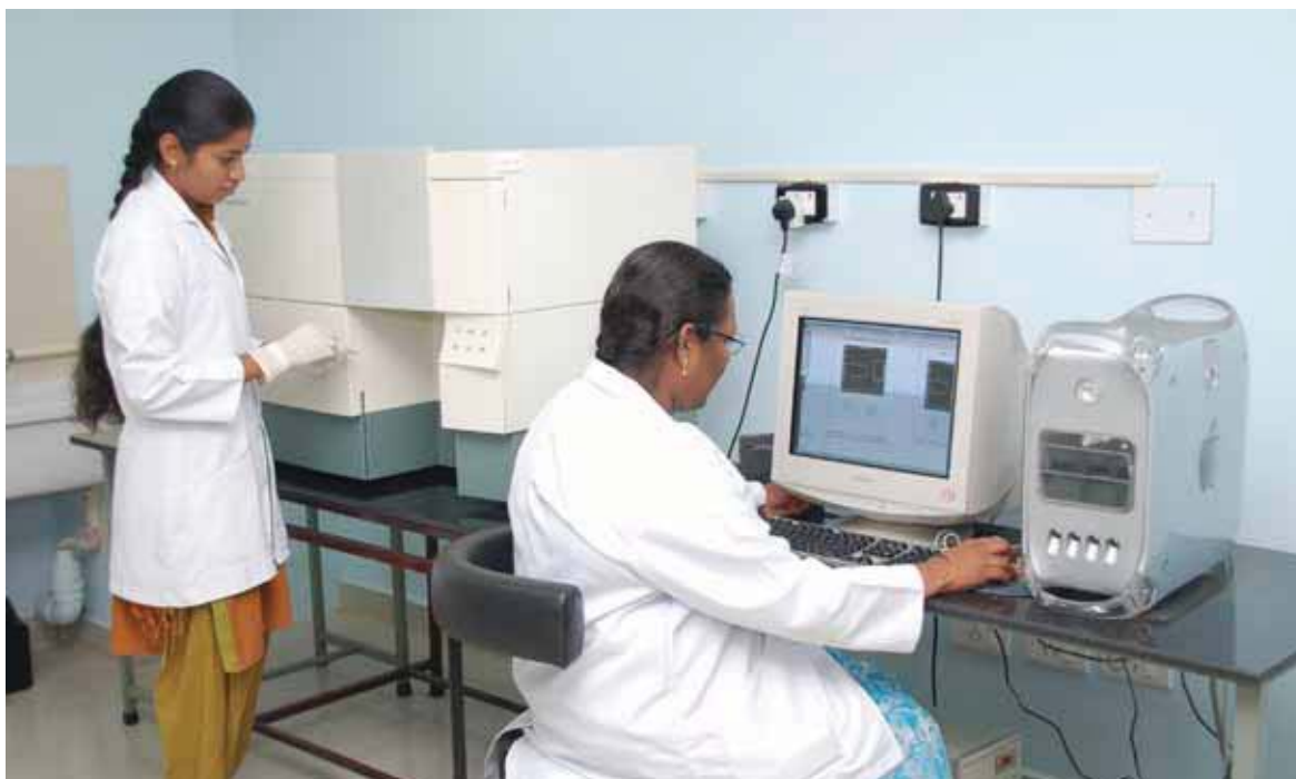
Cytokine analysis using Flow Cytometer
